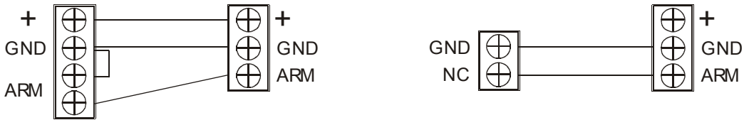
Sensors w/power supply Alarm host zone port Sensors w/o power supply Alarm host zone port
